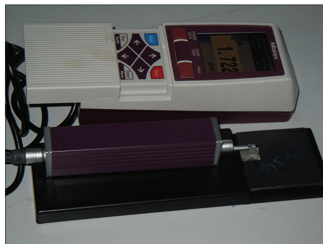
Figure 2: Profilometer – To check surface roughness
